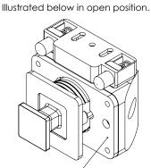
Distance plate to be used by 12 - 13 mm. installation
