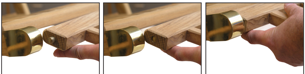
Foot rest plunger in action
