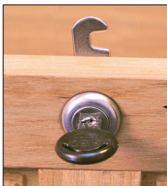
Close up of Cam lock
