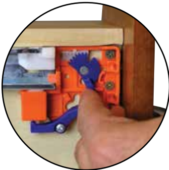
Turn the handle to level the drawer 0-+ 3mm
