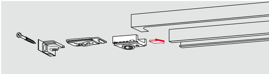
The DORMA RF mechanical hold-open unit ensures that doors are held open at precisely the correct angle – up to approx. 150° – without any fallback.
