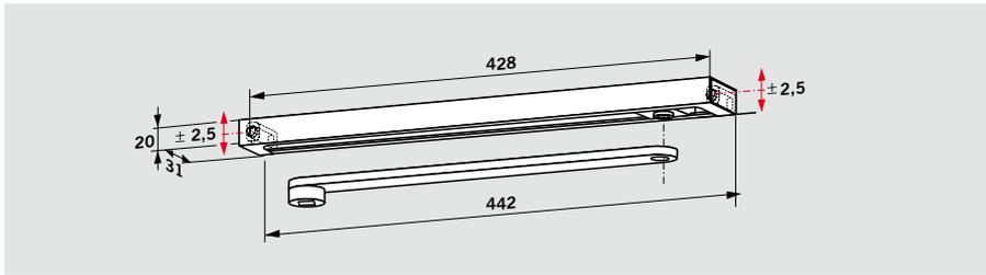
The **DORMA G-N** slide channel assembly comprises the main arm, slide channel, slide block, fixings, screws and end caps. The DORMA G-N slide channel
