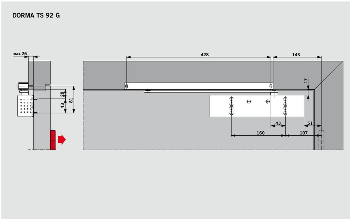
Depending on the structural conditions, the door opening angle with this method of fixing is limited to approx. 120° to 145°. In order to avoid damage to the door or door closer, users are recommended to install a cushioned backstay or a door stop.
