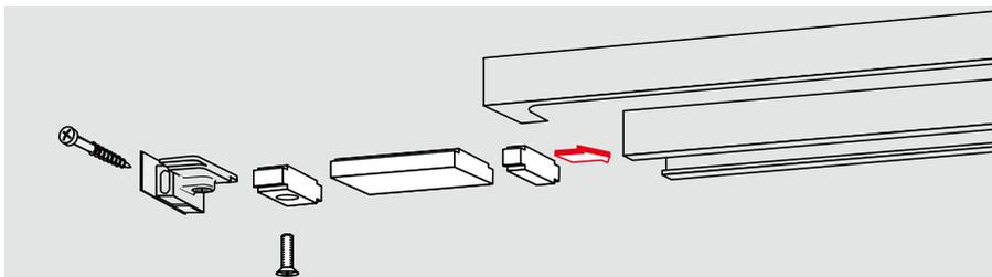
Cushioned limit stay simply slides into the slide channel. Adjustable between 80° and max. 120°. Also suitable for retrofitting.
