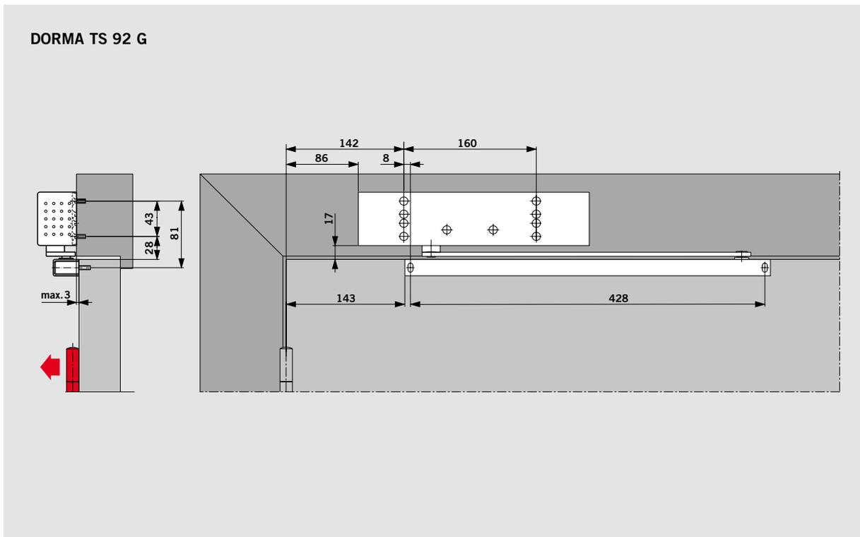
Provided the structural conditions allow, an opening angle of 180° is possible with this method of fixing.
