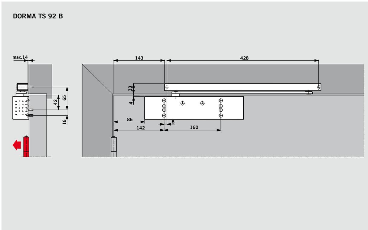
Provided the structural conditions allow, an opening angle of 180° is possible with this method of fixing. In most cases, however, a wall recess will have to be provided for the door closer.
